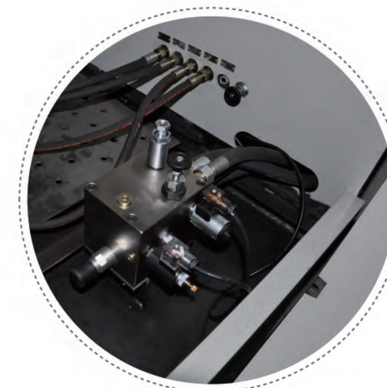
• 正在测试的液压阀 Hydraulic valve that being tested
